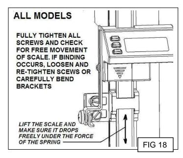
**Note:** If the scale does not slide freely after following the steps in FIG 18, refer to **Trouble shooting** in section 10
