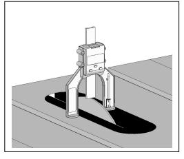
3. Install the plunger and zero the gauge for measuring depths as shown below
