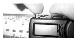
Pull the holder completely out of the protractor
