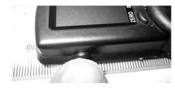
Push on the tab to expose the battery holder
